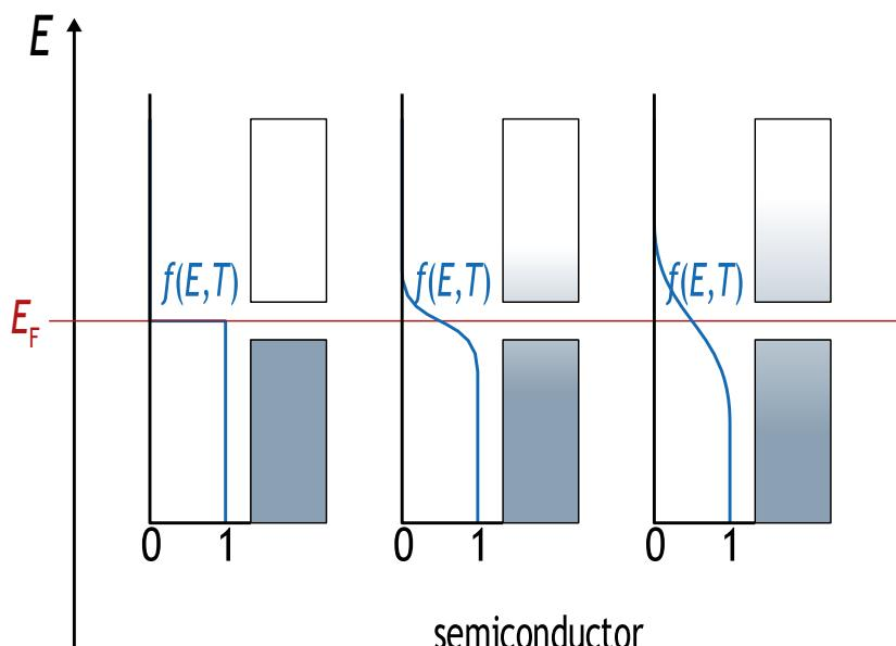
*The density of mobile charge carriers in a pure organic semiconductor is much lower than for pure silicon because the band gap is larger, so at the similar temperatures, the first levels of the conduction bands in organic semiconductors have a lower occupation probability than in pure silicon.*
