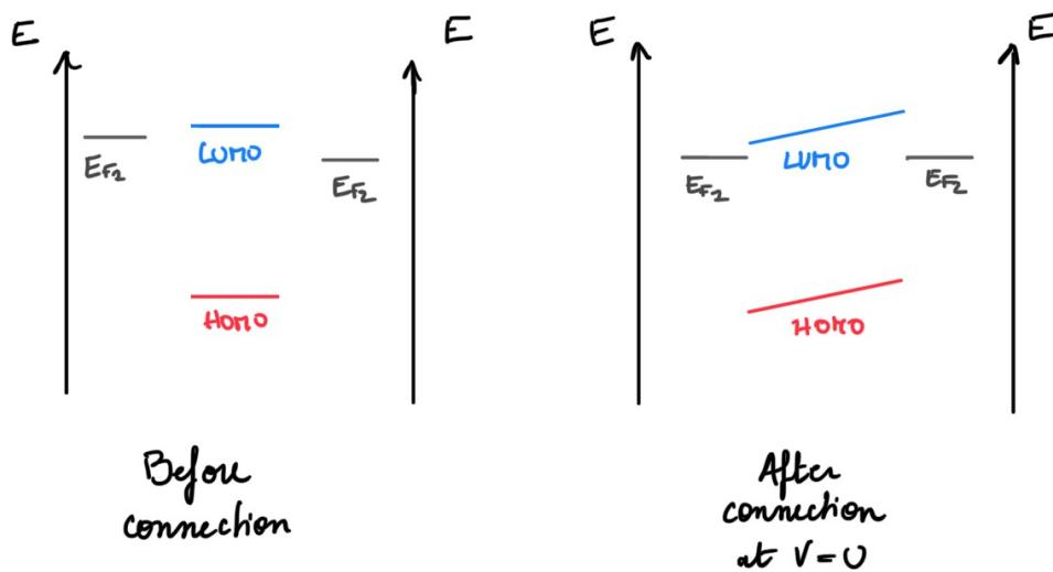
*By choosing electrodes with fermi levels around the LUMO level of the organic semiconductor sandwiched in between, only electrons flow on the LUMO will participates to the current in the device.*
