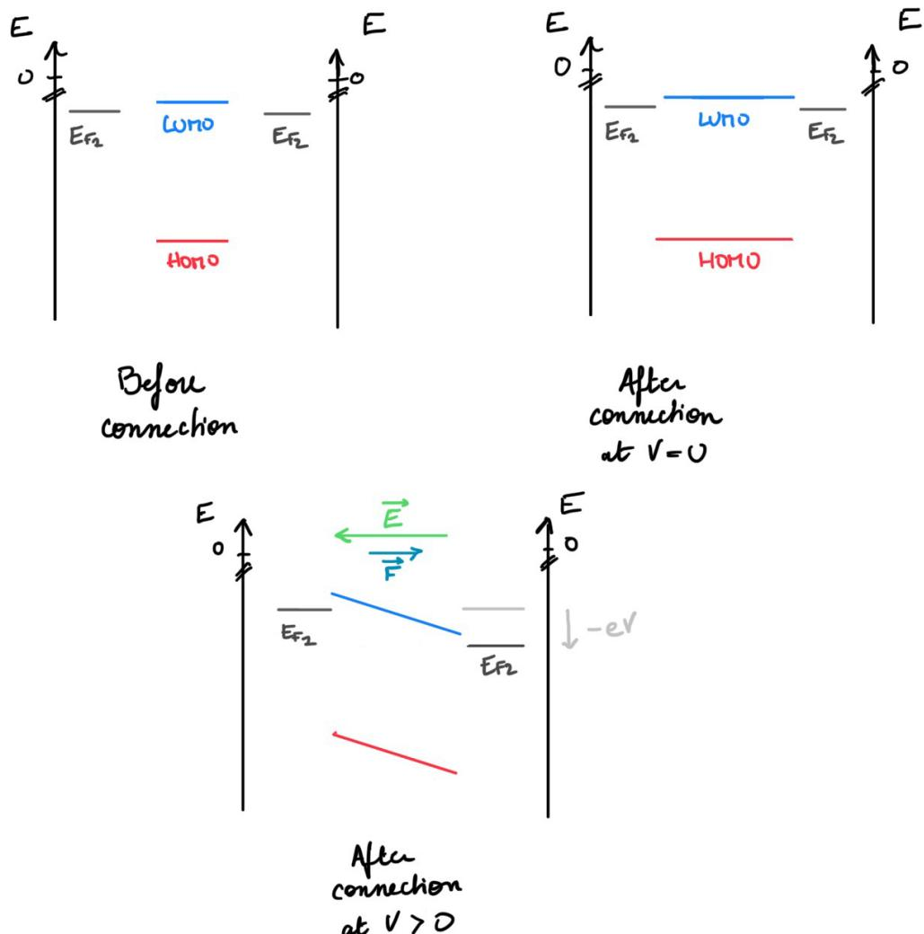
Applying a positive voltage of the right electrode effectively shift its Fermi level of  $qV$  with  $q=-e$  (since electrons are constituting the electrode), so it lowers it. This electrode becomes then effectively less charged (there is less electrons or they are deeper in energy, so require more energy to move) than the left one.
